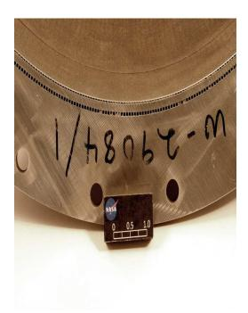
Interim inspection improves the quality of parts with intricate internal features like these fuel channels.
