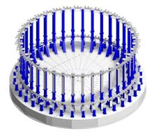
NASA's tooling is made of individual components that are selected, assembled, and adjusted depending on the size and shape of a finished part. CAD models are easily reproduced on the production floor using the modular tooling.
