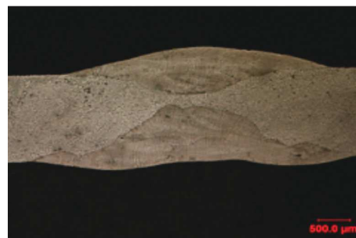
Haynes 230 Super Alloy weld specimens demonstrate the repair of thin-walled pockets. Top photo: Plate 01 Full Penetration. Bottom Photo: Plate 02 Partial Penetration
